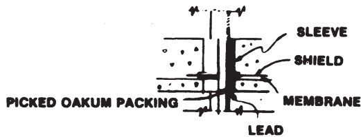
TYPICAL SLEEVE THROUGH FLOOR SLAB WITH MEMBRANE
